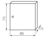
Colour: white Door colour: white Place of assembly: wall mounted Norm: PN-EN 62208 Length [mm]: 485 Width [mm]: 115 Height [mm]: 715
